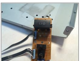
Use a soldering iron to desolder the power switch's terminals and connections. Remove the power switch, replace it, and solder it back together. Repeat these steps in reverse order to put the cassette player back together.
