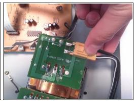
Locate the power cord connection and disconnect it. To remove it, press down on the plastic tab
