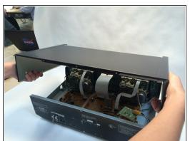
Unscrew the 8mm Phillips head screw from the back of the cassette panel. Remove the cover.
