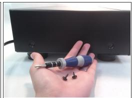
Unscrew the 8mm Phillips head screws from the left and right sides of the cassette player.
