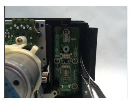
Unscrew all five 7.5mm Phillips head screws from the PCB (printed circuit board) behind the power switch.
