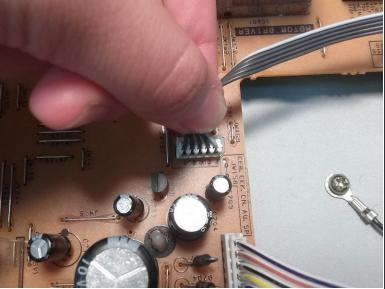
Locate the cords that are connected to the power button. Remove the connection by tugging on the cords gently, releasing them from the main PC board.
