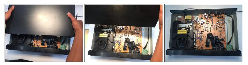
• Remove the top of the CD Player by holding each side of the roof then sliding it away from the front of the CD player.
