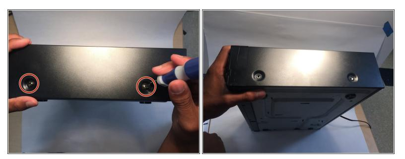
• Remove the two Phillips screws on both sides of the CD Player.
