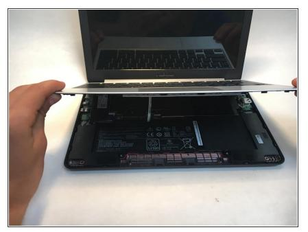
• Slide the plastic opening tool around the length of the keyboard to free it from the laptop. Once the keyboard is free of the computer, lift the keyboard up gently until you can see and reach the two wires attaching it to the computer.
