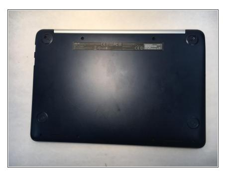
Screw all 1/2 cm screws back into place using the Phillips head #1, and push the plastic sliders back into their slots.
