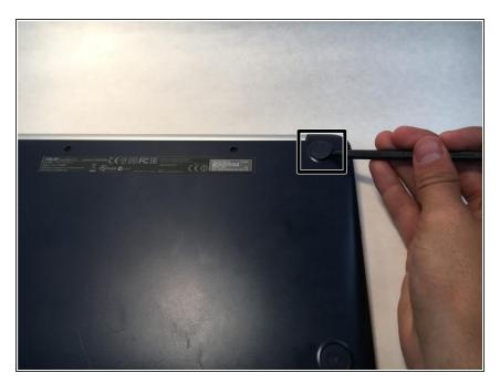
• Then, pull off the plastic sliders on either side of the bottom of the computer using the spludger.
