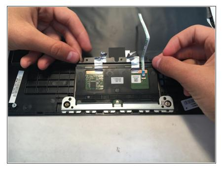
Place new trackpad into slot at an angle. Gently push new trackpad into the slot and press down on it very gently to make sure that it is completely in the slot.
