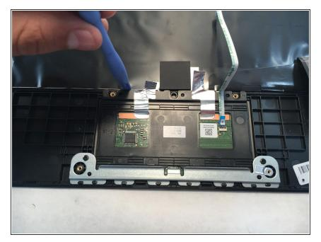
Gently pry up the trackpad with a plastic opening tool. gently tilt the trackpad out of its slot and pull the trackpad out of the keyboard at an angle away from the slot.
