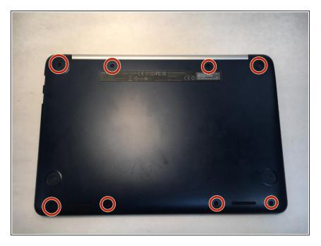
Unscrew all of the screws in the back of the computer. Use a Phillips 1 screwdriver to remove the 8 1/2cm screws.
