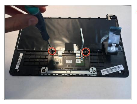
Unscrew the 2/10 cm screws holding the trackpad onto the keyboard using a Phillips head #000 screwdriver.
