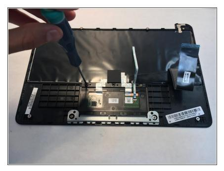
Screw in 2/10 cm screws to hold the trackpad onto the keyboard using a Phillips head #000 screwdriver.
