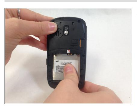
Push down on the silver part of the phone where the battery used to be located. Hold the back of the case to catch it as it comes off.
