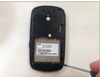
Use a small #00 Phillips-head screwdriver to unscrew all 6 of the 4 mm back screws.
