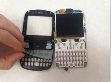
• Lift the keyboard membrane from the bottom and replace it.
