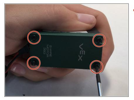
Use a Small Phillips Head Screwdriver to unscrew the four screws from the green casing's corners.
