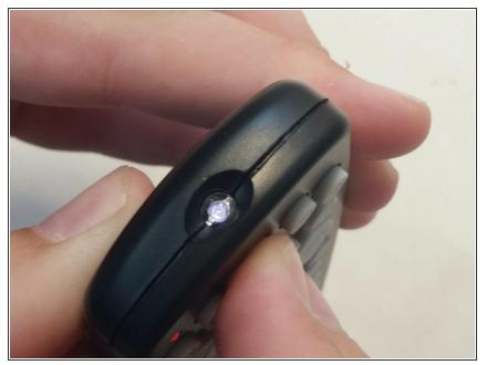
(i) To check if your remote is now working, first make sure the batteries are in correctly. Then, press any button and aim the remote at a smartphone camera. If the LED is working, a red flashing light will be reflected in the camera.
