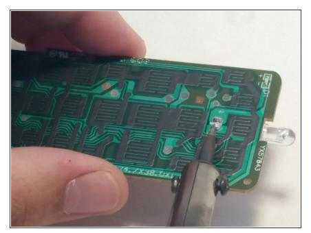
• Desolder the broken LED using a soldering iron and desoldering braid.
