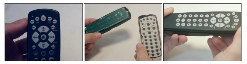
R Make sure the buttons and the circuit board are placed correctly before reassembly.
