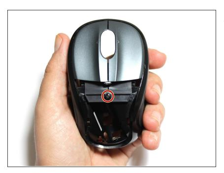
Locate and remove the #0 Phillips screw in the middle of the mouse.
