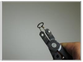
• To remove the Bevel Gear, remove the snap ring wrapped around the base of the gear using Snap Ring pliers.
