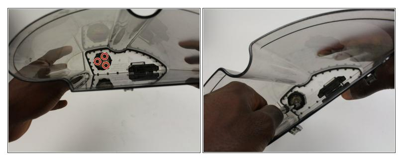
Remove the three 9.5 mm Phillips #1 screws that secure the small circular screen to the bottom of the water reservoir.
