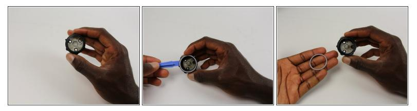
• This circular screen has a rubber "O"-ring around the base. Use the plastic opening tool to pry off the rubber seal. Replace with undamaged seal.
