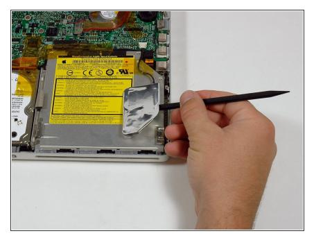
Use a spudger to pry up the PRAM battery from the optical drive.
