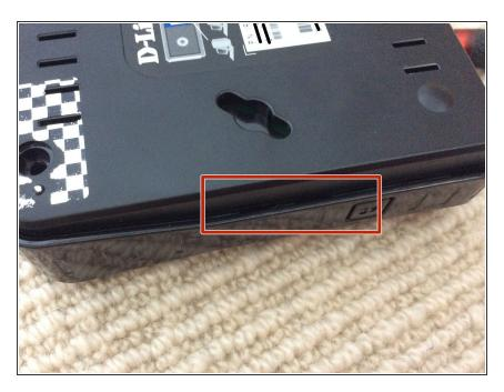
Use a spudger or a flat screwdriver to open it up on both sides.
