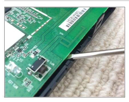
Use a spudger or a flat screwdriver to take out the logic board
