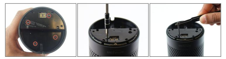
• Remove the four 42.8 mm T10 Torx screws from the bottom of the Echo.
