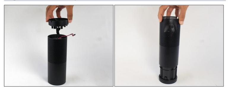
• Remove the plastic plate from the bottom of the device. Then remove the plastic shrouding.
