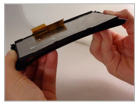
With the screen facing down, firmly grip the sides of the screen frame and pop the screen out.
