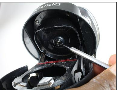
With the Lid still open, locate the Puncture Needle. Insert a paperclip or other small sharp object into the Puncture Needle Holes to remove any debris trapped inside
