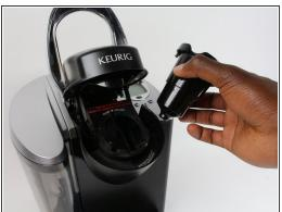
Remove K-Cup Pack Holder Assembly by pinching the left and right sides to release clamp.
