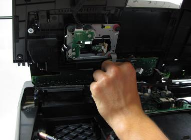
Disconnect the CD drive ribbon cable from the top of the device.
