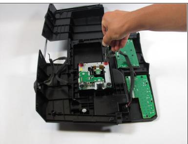
Use a Phillips #2 screwdriver to unscrew the four 1/2 inch screws.
