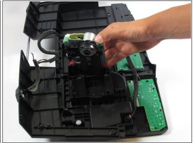
• Firmly grab and lift the CD drive from its plastic compartment to remove it.
