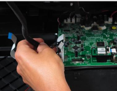
Disconnect the antenna cables.
