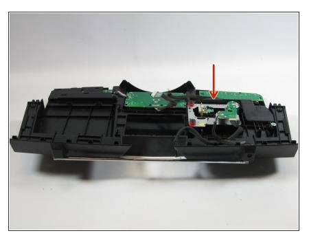
Flip the top and locate the CD module on the right side.
