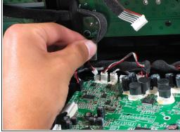
Disconnect the remaining cables from the motherboard.
