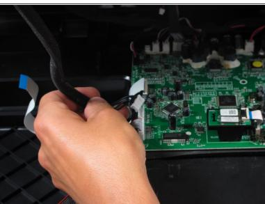
Disconnect the antenna cables.
