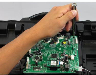
Remove the five 1/2inch screws from the motherboard using a Phillips #2 screwdriver.
