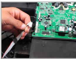
• Remove the following 2 cables from the left side of the board.
