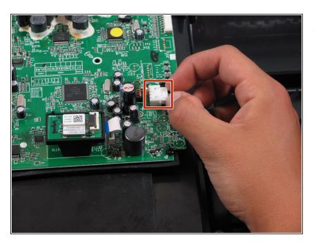
Remove the final cable on the bottom right side of the motherboard.
