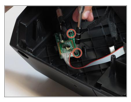
Use a Phillips #2 screwdriver to unscrew the two 1/2 inch screws
