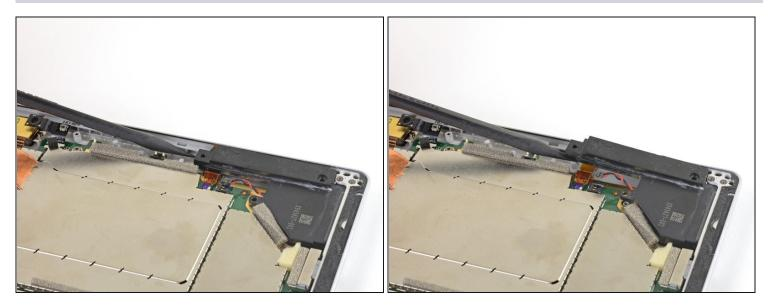
• Use a spudger to lift up the narrow section of the speaker box until you can grip it with your fingers.
