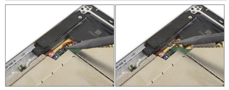
• Gently lift the speaker wire connector straight up with the pointed end of a spudger to disconnect it from the motherboard.
