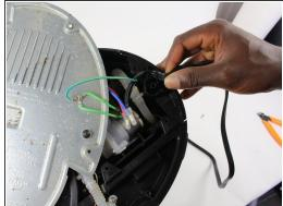
Unwind the Power Cord from the wire channel
