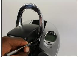
Locate and remove the two 9.5 mm Torx T15 screws on both sides of the handle.
