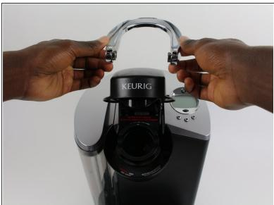
Remove the broken handle and replace with the new one
