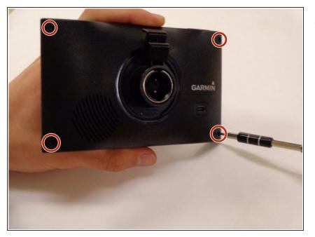
Using a T5 Torx screwdriver, remove four 6 mm screws from the four corners of the back of the device.
