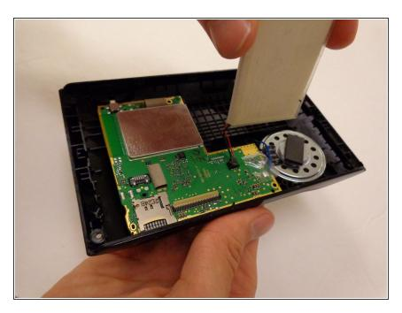
Pull the battery-motherboard connector away from the motherboard.
