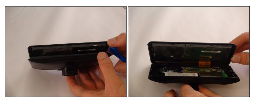
• Carefully pull apart the device by opening it up on the opposite side of the nameplate.
