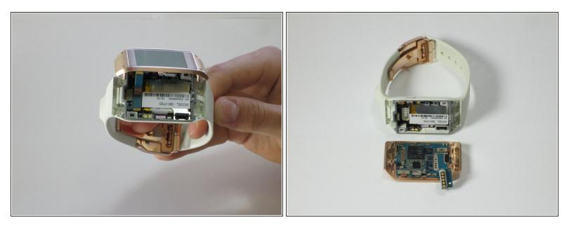
(i) After separating the LCD/motherboard from the actual watch itself, the watch should be in two separate pieces.
