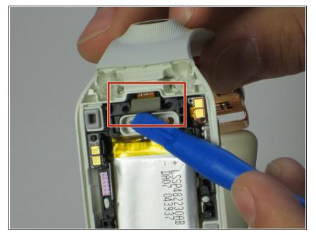
• Loosen the camera ribbon so it will easily pass through the watch body.
