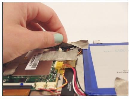
• Gently peel all of the tape that is covering the cable connections going to and from the cameras. Set the tape aside for later reassembly.
