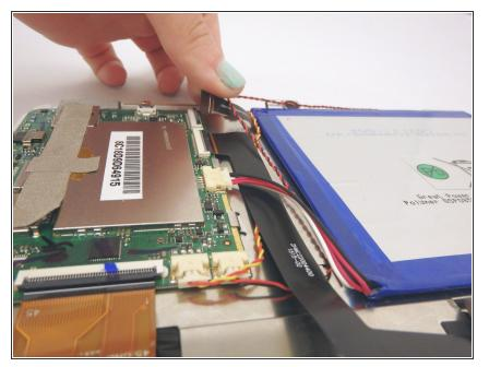
Gently pull camera connector ribbon by hand until it separates from connector.
