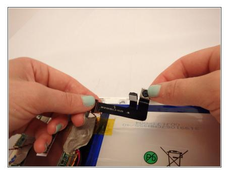
• Remove connector ribbon and cameras from device casing.
