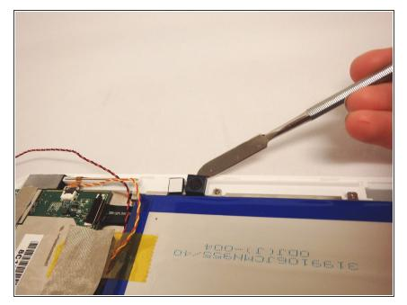
Using metal spudger tool, gently pry the rear-facing camera from the adhesive.
