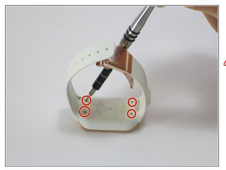
Use a T5 Torx screwdriver to remove the **four** 4.0 mm screws on the back of the device.
