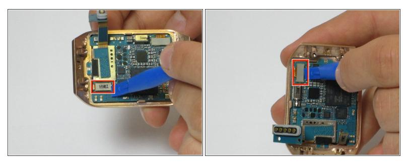
• On the display, use a plastic opening tool to lift up the two ribbon cables the motherboard.
