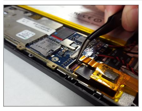
• Lift up on the small black tab to unlock the LCD screen flex ribbon cable using the tweezers.
