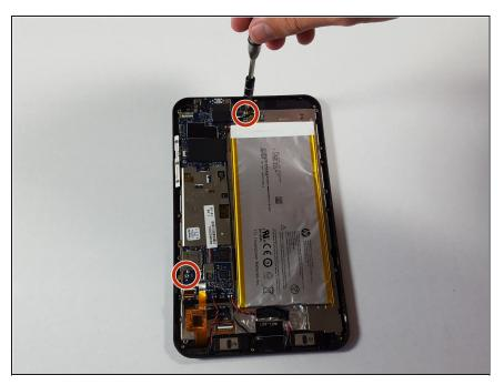
Remove the two Phillips using the screwdriver with a PH00 Phillips head.
