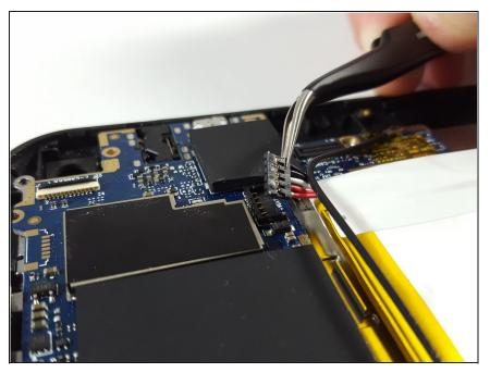
• Carefully remove the battery connector from the system board using the tweezers.
