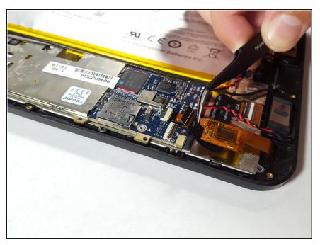
Carefully remove the LCD screen flex ribbon cable from the system board using the tweezers.
