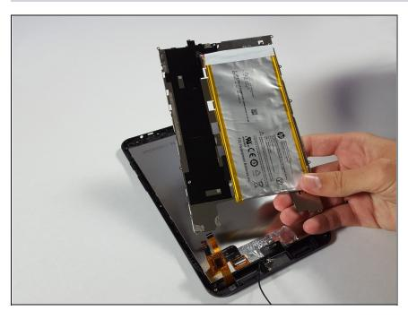
• The battery can now be removed from the device.
