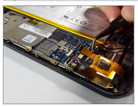
Carefully remove the USB flex ribbon cable from the connection point on the system board using the tweezers.
