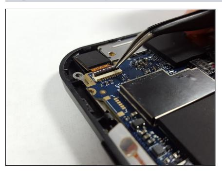
Lift up on the small black tab at the connection point to unlock the flex ribbon cable using the tweezers.
