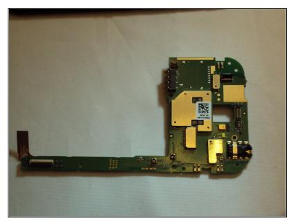
• Remove the motherboard from the casing.
