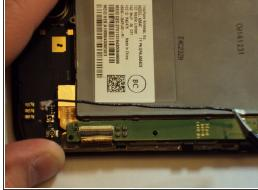
Using tweezers, carefully detach the antenna from the motherboard.
