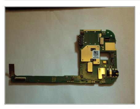
Remove the motherboard from the casing.
