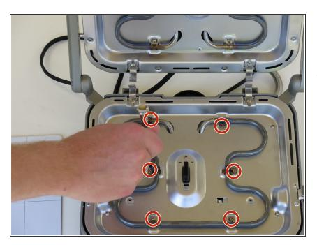
Remove the six 5.5mm Phillips #2 screws that secure the bottom heating coil to the device.
