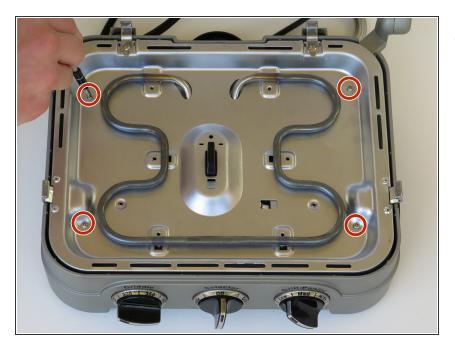
Remove the four 30 mm Phillips #2 screws that secure the bottom heating apparatus.
