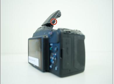
Unscrew the two black, 4mm screws with a Philips 000. (There should be one screw on each side of the camera).
