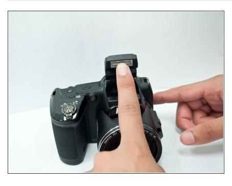
Push the flash inward to pop the flash out of its front case. Since the back case is removed, the flash should pop out from the back.
