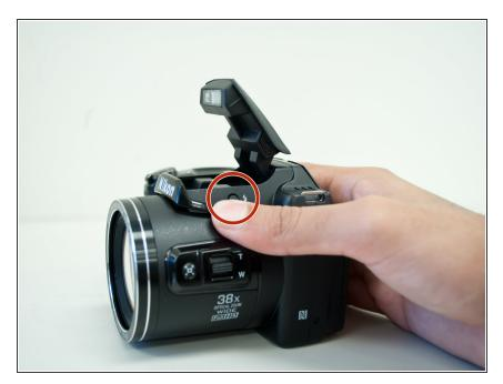
Press the flash button on the side of the camera to allow the flash to spring upward.
