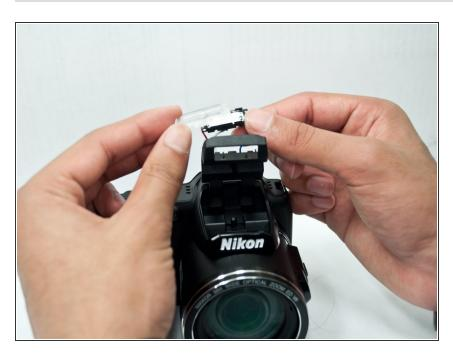
The see-through protective flash covering is stuck on to the flash with thin, double-sided tape. Pull apart the two components to access the flash.
