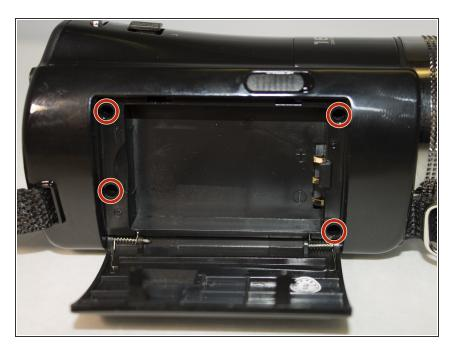
With the battery door open, carefully remove all four 5 mm Phillips #1 screws.
