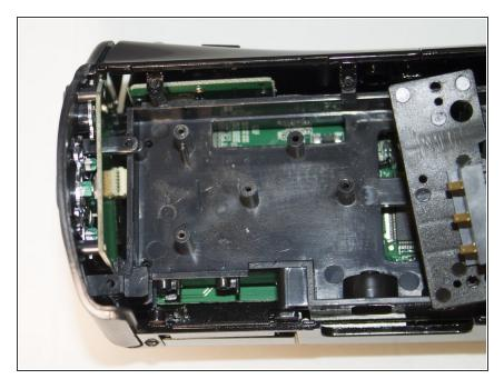
Apply pressure to the back panel (away from the camera) to remove.
