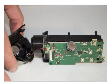
Pull forward on the lens casing to remove it. The cord connecting the light to the motherboard should still be attached.
