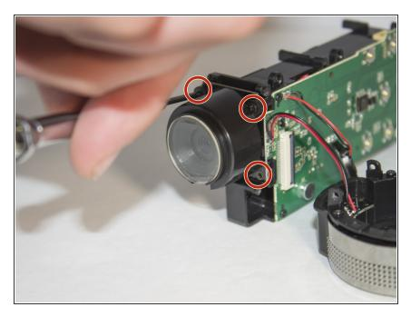
Unscrew the three 4 mm Phillips #1 screws holding the plastic lens holder.
