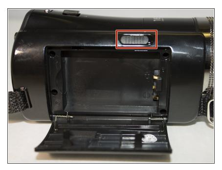
Slide the battery eject button open to release the battery door.
