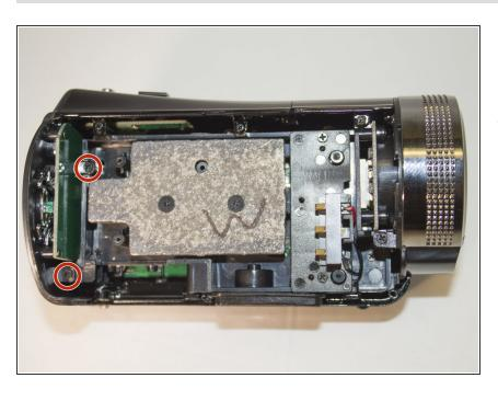
Remove the two 4 mm Phillips #1 screws holding the back panel in place.
