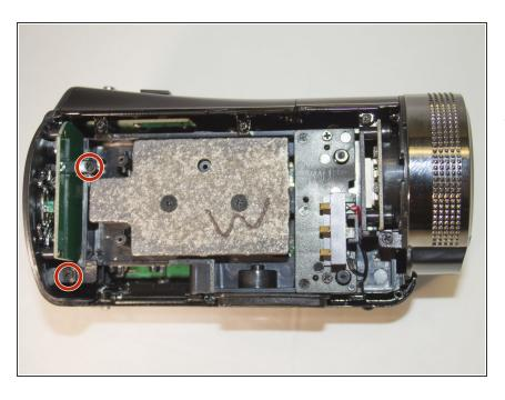
Remove the two 4 mm Phillips #1 screws holding the back panel in place.
