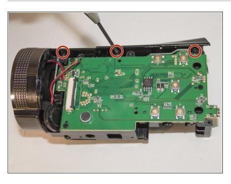
Remove the three 4 mm Phillips #1 screws holding the top panel in place.
