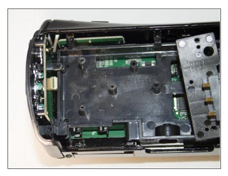
Apply pressure to the back panel, pulling away from the camera to remove it.
