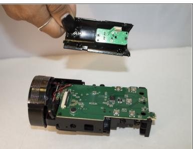
Push upward on the top panel to remove it from the body of the camera.
