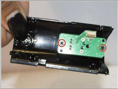
Remove the two 4 mm Phillips #1 screws holding the circuit board in place.
