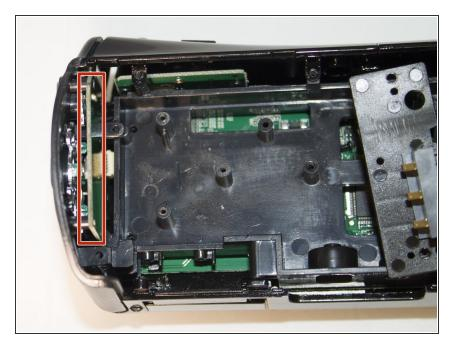
Remove the back panel away from the camera by applying pressure to it.
