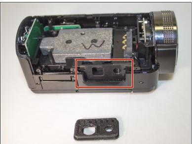
Apply pressure upwards to remove the tripod clip.
