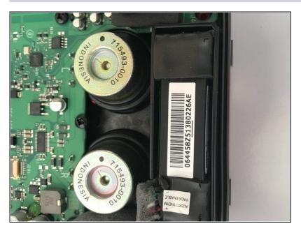
Put back the sponge cover, it is necessary to avoid vibrations and to keep the thing firmly in place.
