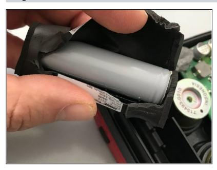
Partially cut the battery cover on the side paying attention to do not damage the circuit or the battery. Cut the cover just enough to remove it, try to not damage it too much as it is going to be reused.
