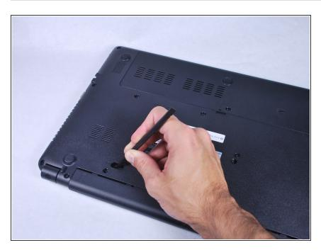
To release the battery, depress the battery release with a nylon spudger. Hold the latch down and slide it over.
