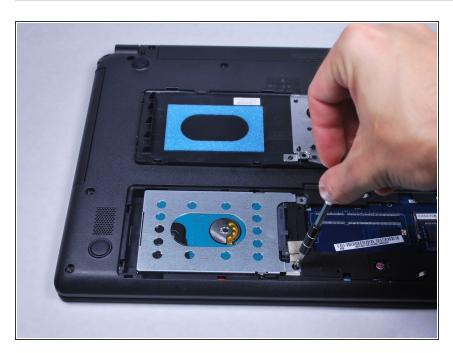
Use a PH0 Phillips screwdriver to remove the screw securing the hard drive.
