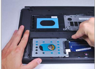
Use a nylon spudger to slightly pry up the hard drive near the screw holes.
