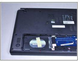
Grab hold of the plastic tab and pull the hard drive away from the connectors. This will release the hard drive.
