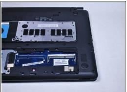
Rotate the RAM sticks up and slide the RAM out.
