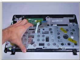
Use the plastic opening tool to slide the metal part out to release it from the retaining tabs.
