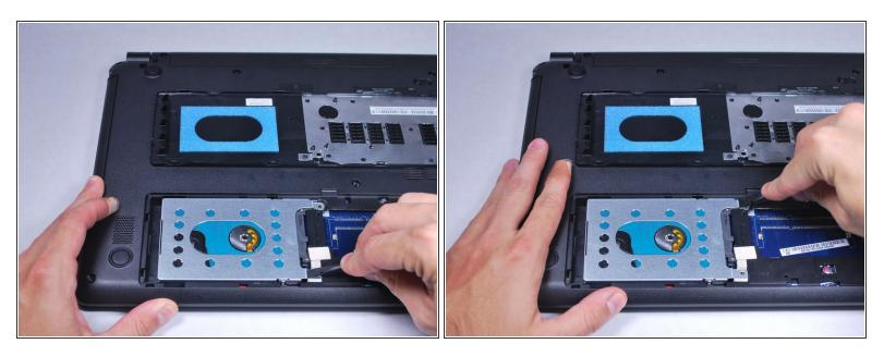
• Use a nylon spudger to slightly pry up the hard drive near the screw holes.
