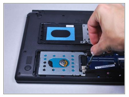
Use a PH0 Phillips screwdriver to remove the screw securing the hard drive.
