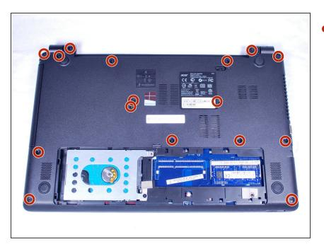
Remove the fourteen M2.5x8 screws highlighted in the picture with a PH0 Phillips screwdriver.
