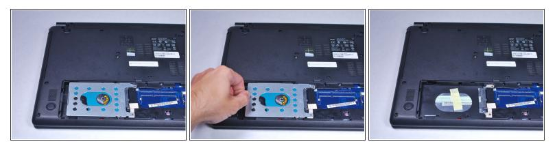
• Grab hold of the plastic tab and pull the hard drive away from the connectors. This will release the hard drive.
