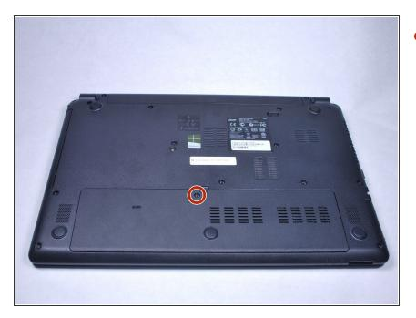
Remove the M2.5x8 screw with a PH1 screwdriver.
