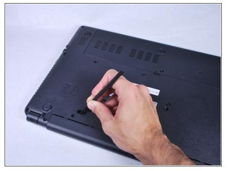
To release the battery, depress the battery release with a nylon spudger. Hold the latch down and slide it over.
