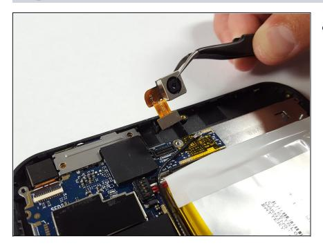
Remove the back facing camera with the tweezers.
