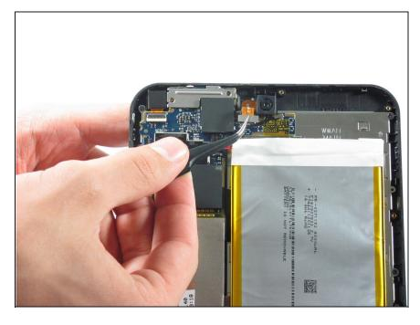
• Carefully pry up the gray metal piece on the end of the flex ribbon cable using tweezers.
