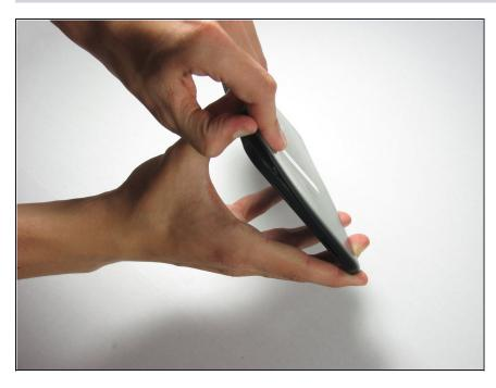
• Use your nail or a spudger to pry the back cover off of the device.
