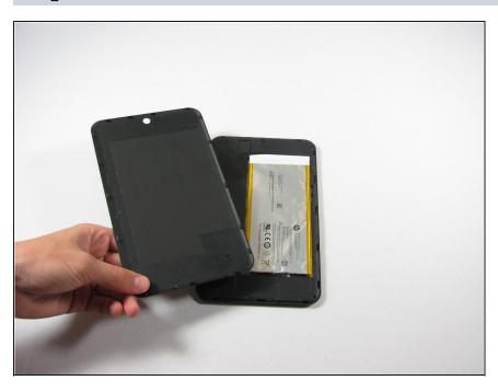
Slide your finger around the rest of the back cover, lifting it completely off of the device.
