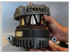
Once the pulley is removed, separate the rotor and stator. The stator is the piece with copper windings.
