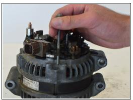
Use a Philips #2 Screwdriver or a 7.5mm socket driver to unscrew the 4, 7.5mm bolts running along the outer perimeter of the alternator
