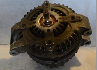
Once the nut is off, you can then remove the pulley.
