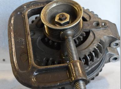
Use a c-clamp or another fixture to hold the pulley in place
