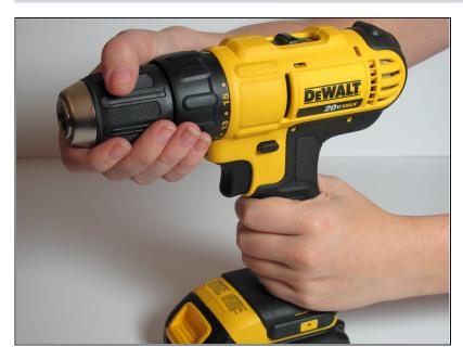
Loosen the chuck until it is all of the way open.
