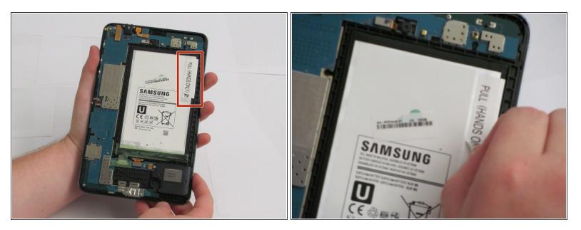
Peel the sticker, reading "PULL (HANDS ONLY)," off of the battery starting at the detachable corner.
