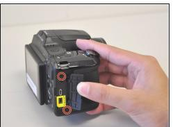
• Unscrew all eight black, 4mm screws with a Philips 000. (The top-most screw shown in the third image can be accessed by lifting the cover flap off.)
