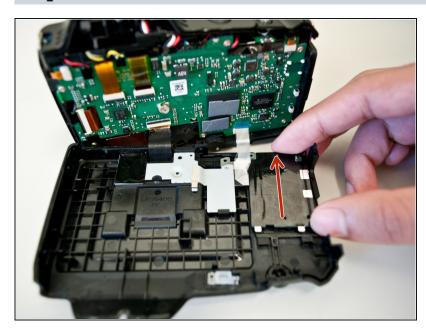
Slide off the button panel in the marked direction.
