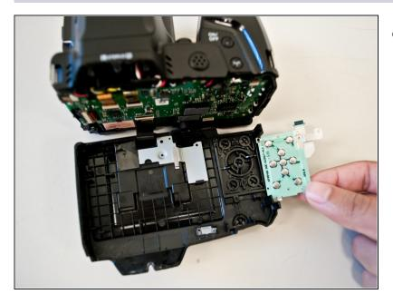
Flip to the front side of the button panel to access the button sensors.
