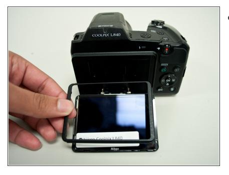
The front cover comes off easily once the back cover is removed in Step 4.
