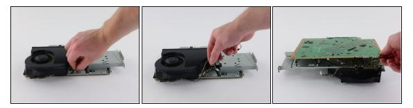
Remove the fan wire from its plug on the top metal casing.
