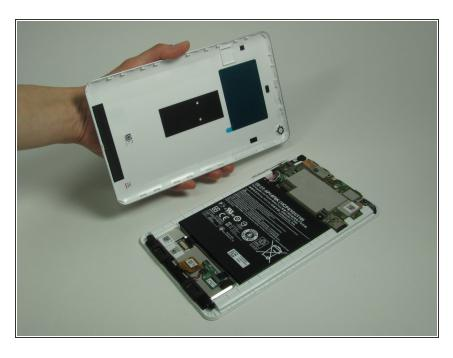
Separate the rear case and place the tablet face side down. To reassemble your device, follow these instructions in reverse order.
