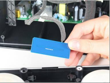
Gently remove the wireless card located at the bottom of the front speaker panel by pulling up and out with your index finger and thumb. To reassemble your device, follow these instructions in reverse order.
